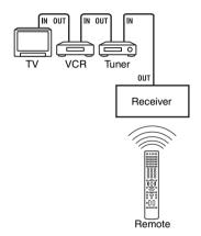
The remote sensor on this receiver receives remote codes the same way as the remote sensor on the CONTROL S IN component. This is useful if you place the other component away from this receiver.
